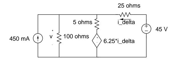
3. **Thevenin equivalent with dependent and independent sources** Find the thevenin equivalent of the following circuit with respect to terminals ab.
