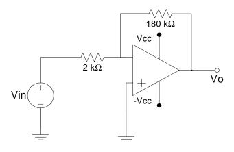
The inverting amplifier in the circuit at left has an input resistance R<sub>i</sub> of 500 k $\Omega$ , an output resistance R<sub>o</sub> of 5 k $\Omega$ , and an open loop gain A of 250,000. Assume that the amplifier is operating in its linear region (i.e., ignore the rails).
