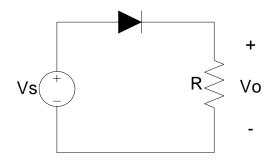
Let Vs = 1 V, R = 1 k $\Omega$ . Use the load-line method to find Vo at left.
