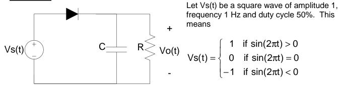
With Vo(t=0)=0, R = 10 k $\Omega$  and C = 50  $\mu$ F, sketch Vo(t) for t = 0 to t = 3 seconds.
