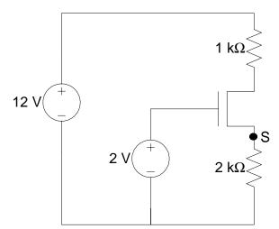
$W/L\mu_N C_{\text{OX}} = 200 \ \mu\text{A}/\text{V}^2, \ V_{\text{TH}(N)} = 1 \ \text{V}, \ \lambda = 0 \ \text{V}^{\text{-1}}.$
