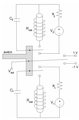
Let  $V_1 = V_2 = 10 \text{ V},$   $C_1 = C_2 = 145 \text{ pF},$   $R_{\text{coil}} = 20 \text{ k}\Omega,$   $R_1 = R_2 = 10 \text{ k}\Omega.$ Coil holds the switch in place as long as it voltage exceeds 5 V.
