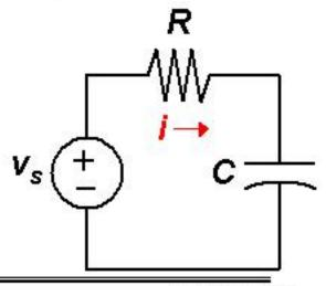
The natural response of an RL or RC circuit is its behavior (i.e. current and voltage) when stored energy in the inductor or capacitor is released to the resistive part of the network (containing no independent sources).
