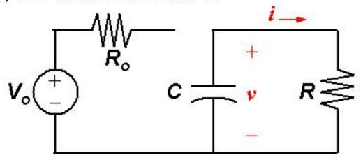
Applying KCL to the RC circuit:
