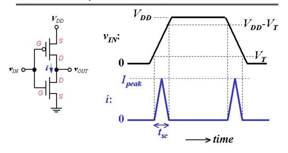
Energy consumed per switching period:  $E_{dp} = t_{sc} V_{DD} I_{peak}$
