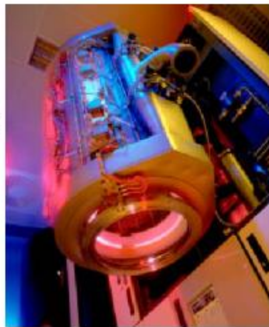
ASM A412 batch oxidation furnace
