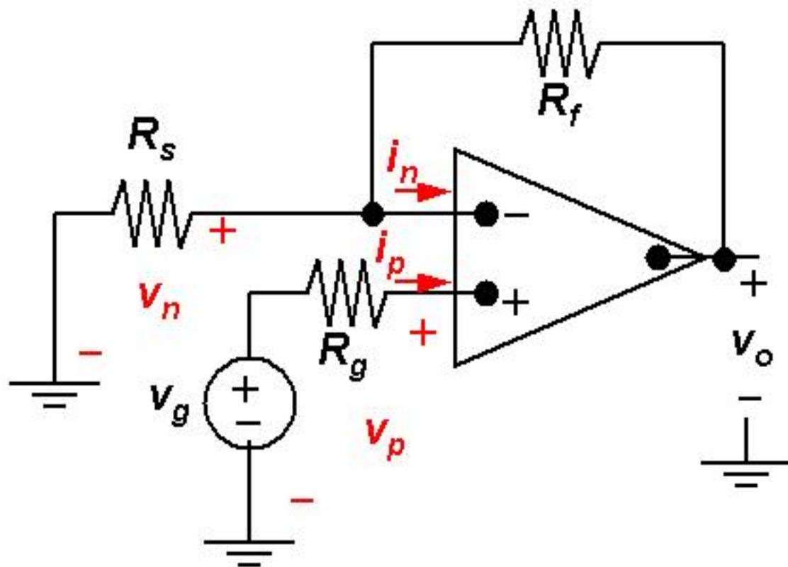
$$v_o = \frac{R_s + R_f}{R_s} v_g$$
