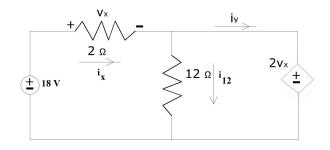
Applying KVL around the periphery of the circuit, we have  $-18 + v_x + 2v_x = 0$ which yields  $v_x = 6 V$ . Then we have  $v_{12} = 2v_x = 12 V$ . Using Ohm's law we obtain  $i_{12} = \frac{v_{12}}{12} = 1 A$  and  $i_x = \frac{v_x}{2} = 3 A$ . Then KCL applied to the node at the top of the  $12\Omega$  resistor gives  $i_x = i_{12} + i_y$  which yields  $i_y = 2 A$ . With the sign conventions as shown in the figure, the power delivered to the 18
