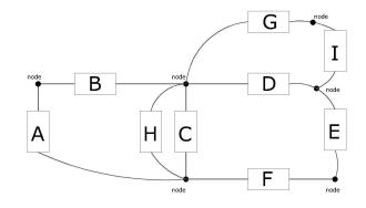
A node is a point at which two or more current elements are joined together. All points connected by ideal conductors are considered to be a single node. There are 6 nodes in this circuit as indicated in the figure above.
