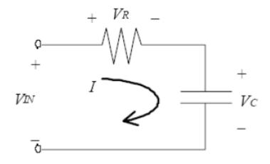
a) Assume the voltage across capacitor (capacitance C) is  $V \sin(\omega t + \theta)$ . Find the current through the capacitor. (Hint: read the lab)
