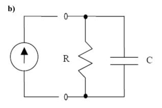
**3.** An RC (resistor + capacitor) circuit will have an exponential voltage response of the form v(t) =  $A + B e^{-t/RC}$  where A and B are constants that express the final voltage and the difference between the initial voltage and the final voltage, respectively.
