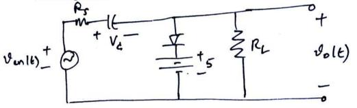
This is exactly like the circuit of Figure 10.33 of the text, except that the DC voltage source has been flipped. Note that we could also have attempted to realize this by instead using a Zener diode with a breakdown voltage of 5V as in the following circuit:
