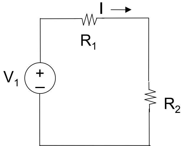
$$I = \frac{V_1}{R_1 + R_2}$$
