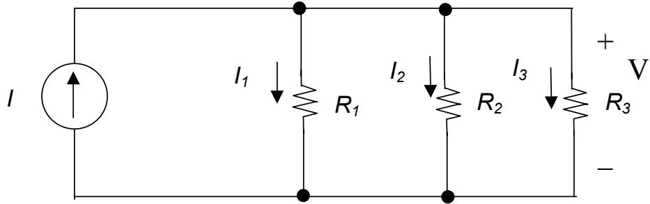
$$V = \frac{I}{\left(\frac{1}{R_1}\right) + \left(\frac{1}{R_2}\right) + \left(\frac{1}{R_3}\right)}$$
