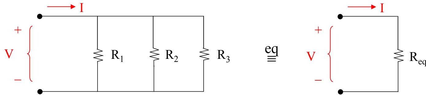
**Equivalent conductance of resistors in parallel is the sum of their individual conductances**
