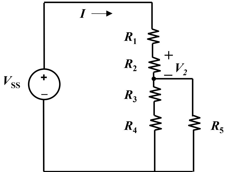
$$V_2 \neq \frac{R_2}{R_1 + R_2 + R_3 + R_4} \cdot V_{SS}$$
