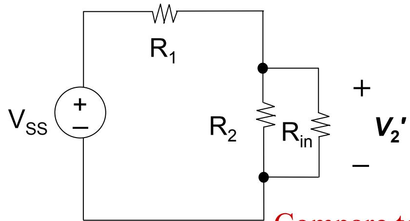
$$V_2 = V_{SS} \left[ \frac{R_2}{R_1 + R_2} \right]$$
