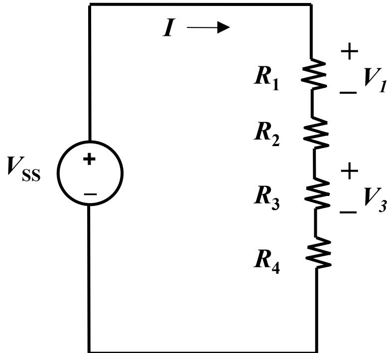
$$I = V_{SS} / (R_1 + R_2 + R_3 + R_4)$$
