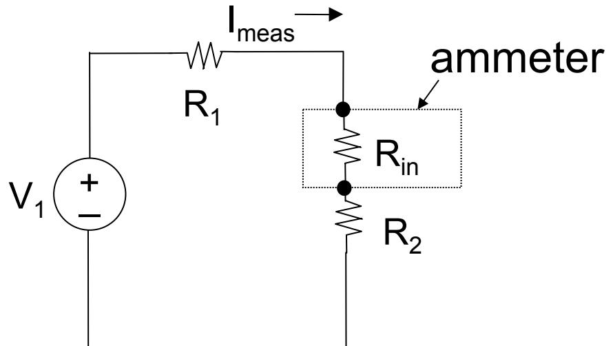
$$I_{\text{meas}} = \frac{V_1}{R_1 + R_2 + R_{\text{in}}}$$
