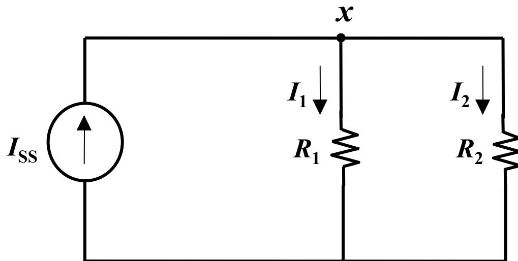
$$V_x = I_1 R_1 = I_{SS} R_{eq}$$
