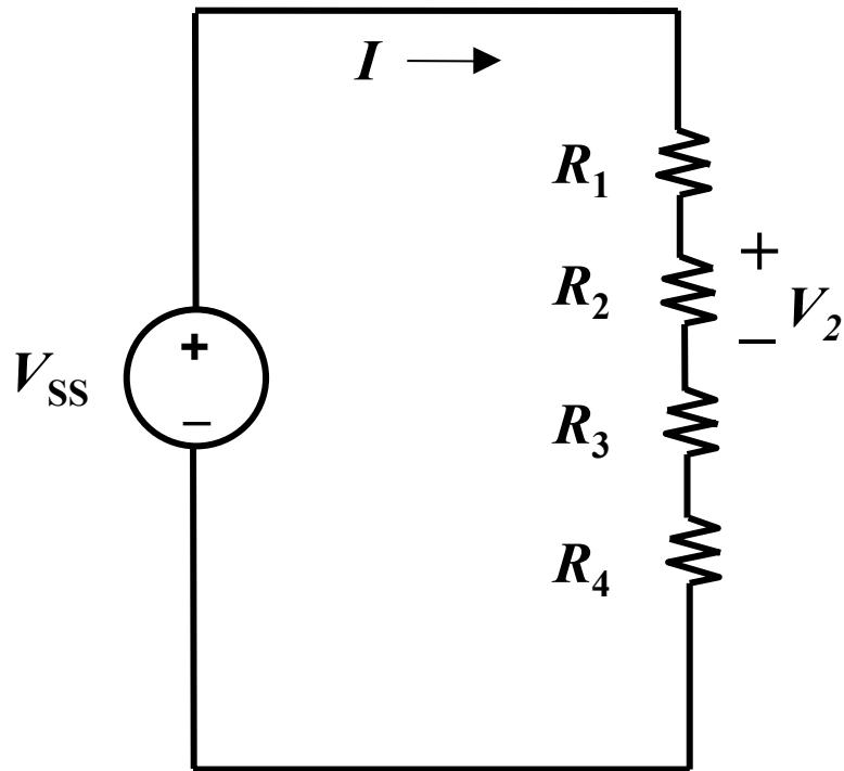
$$V_2 = \frac{R_2}{R_1 + R_2 + R_3 + R_4} \cdot V_{SS}$$
