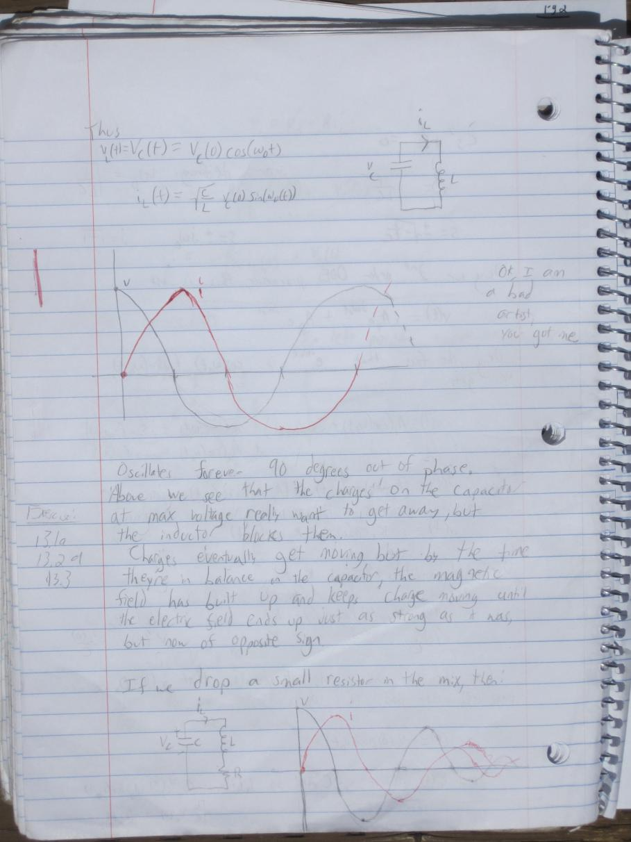
Sinusoid slowly dies. If R gets big we see an abrupt qualitative change. At some point, damping becomes so strong that oscillations clease completely. High 1 No Oscillation Com Still overshoot How do we show this? 2. Write ODE for whole circuit
