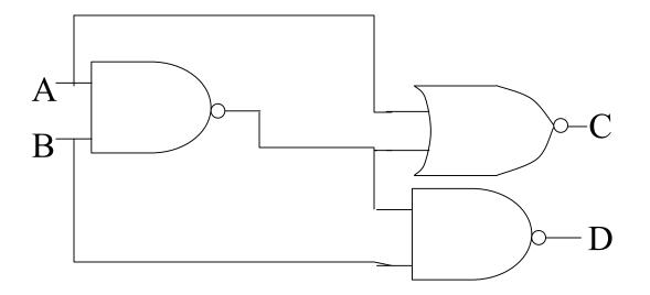
Every node in any circuit (such as the internal circuit of a NAND gate) has capacitance and all interconnects have resistance. Thus it takes time to charge these capacitances.
