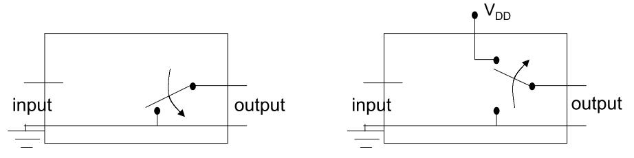
• A PMOS transistor is just the ticket. It is precisely as ideal a switch for connections to high as NMOS transistors are for connections to low.
