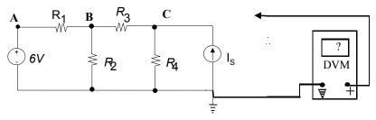
Thus we can connect the + lead of the DVM to point (Node) A and call the potential of point A " $V_A$ ", similarly at points (Nodes) B, C.
