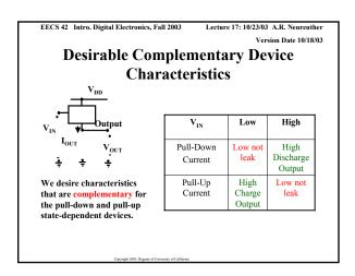
EECS 42 Intro. Digital Electronics, Fall 2003 Lecture 17: 10/23/03 A.R. Neureuther Version Date 10/18/03 Designing the Complementary Device Into This Make This 100 100 I<sub>OUT</sub>(µA  $I_{\text{OUT}}(\mu A)$ 60 60 The curve sets are very similar but have two key changes. The creation of current with input State (VIN) is reverse ordered (and also shifted). The dependence on  $V_{OUT}$  is reversed in sign and shifted by  $V_{\rm DD}$
