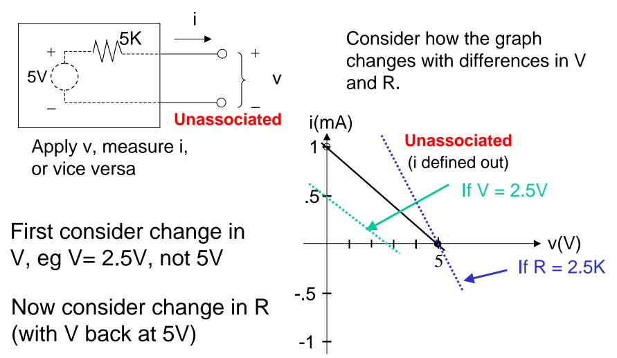
Clearly by varying V and R we can produce an arbitrary linear graph ... in other words this circuit can produce *any* linear graph
