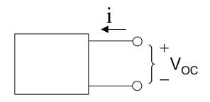
2a) If we short the output clearly I =  $-V_T/R_T$  thus  $R_T$  is the ratio of  $V_{OC}$  to  $-i_{SC}$ , the short-circuit current
