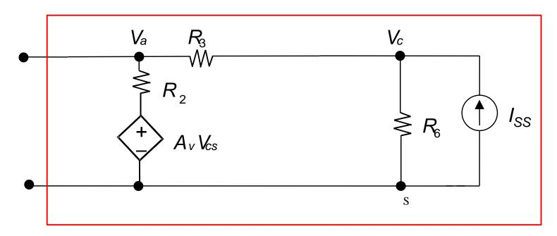
With method 2 we first find open circuit voltage  $(V_T)$  and then we "measure" input resistance with source  $I_{SS}$  turned off.
