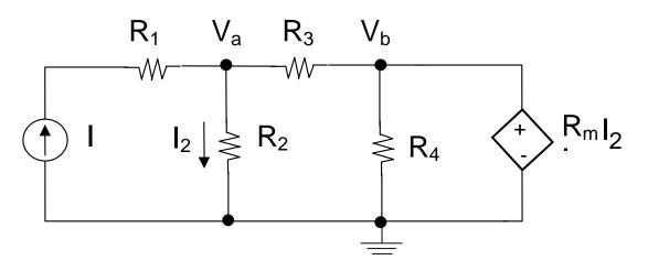
Standard technique, except an additional equation is needed if the dependent variable is an unknown current as here. Note Vb is redundant.
