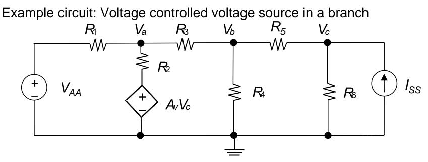
Write down node equations for nodes a, b, and c.
