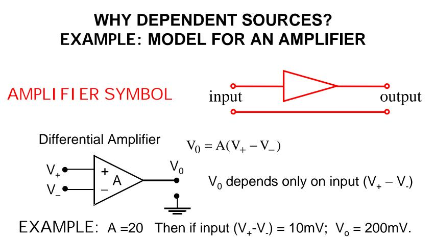
An actual amplifier has dozens (to hundreds) of devices (transistors) in it. But the dependent source allows us to model it with a very simple element.
