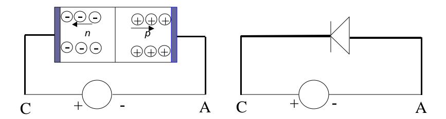
This is the direction of almost zero current flow. The + charges are just pulled away from the junction, and so are the - charges. Essentially zero conduction.
