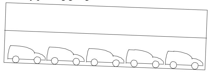
If the lower floor is full and top one is empty, no traffic is possible. Analog of an insulator. All electrons are locked up.
