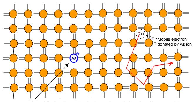
Immobile (stuck) positively charged arsenic ion after 5<sup>th</sup> electron left
