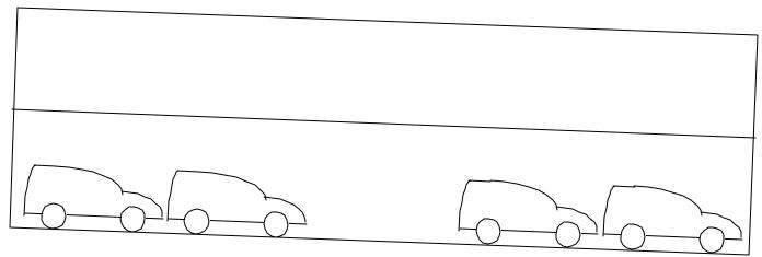
If a car is removed from the lower floor, it leaves a HOLE which can move. Conduction is possible. *Analog to P-type semiconductor.* (Acceptors are added to the crystal, "consuming" bonding electrons, creating free holes).
