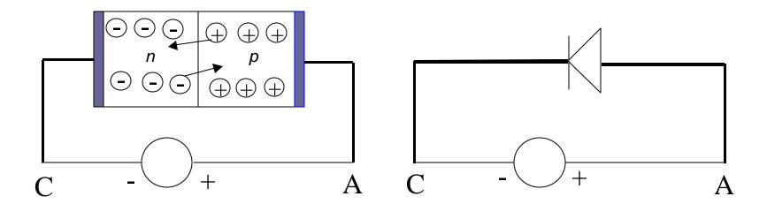
This is the direction of easy current flow. + charges flow to meet up with – charges. Essentially unlimited conduction.
