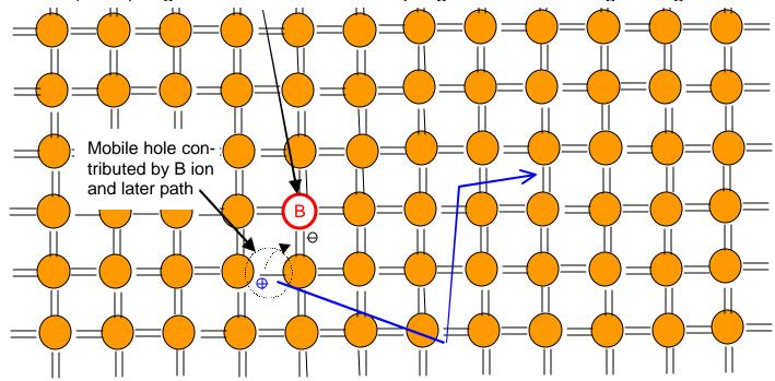
The "hole" which is a missing bonding electron, breaks free from the B acceptor and becomes a roaming positive charge, free to carry current in the semiconductor. It is positively charged.
