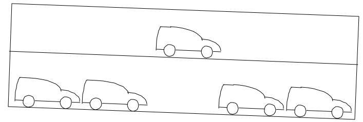
If one car is moved upstairs, it can move AND THE HOLE ON THE LOWER FLOOR CAN MOVE. Conduction is possible. Analog to warmed up semiconductor. Some electrons get free (and leave "holes" behind).
