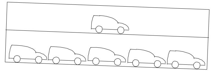
If an extra car is "donated" to the upper floor, it can move. Conduction is possible. *Analog to N-type semiconductor*. (An electron donor is added to the crystal, creating free electrons).
