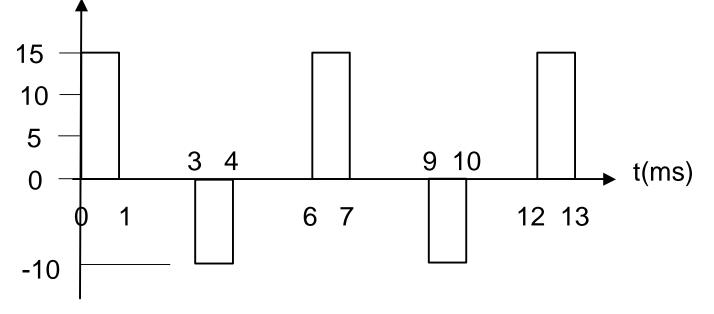
Lets average over a 6ms interval (that is the period) Now the average power is (15 - 10)/6 mW or 5/6 mW.
