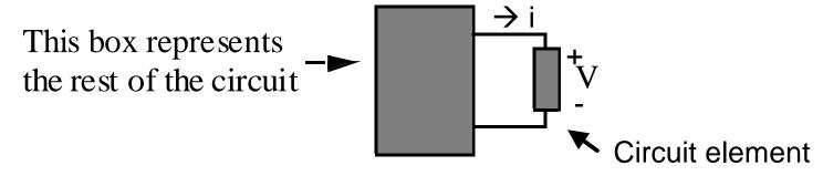
For positive current and positive voltage, positive charge "falls down" a potential "drop" in moving through the circuit element: it *absorbs* power
