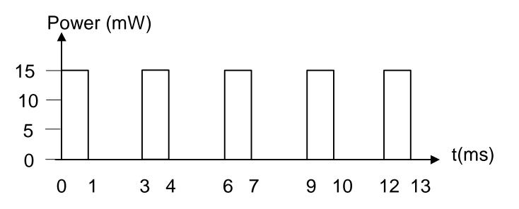
Lets average over the 3ms period of the waveform: Clearly the average power is 15/3 mW or 5mW.
