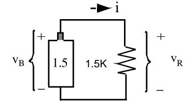
A) For Resistor:  $P = i v_R$ (because we are using + (because we are using  $v_R$  "associated reference directions") Hence, P = i  $v_R$  = +1.5mW
