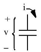
but dq = C dv. (We are using small q instead of Q to remind us that it is time varying . Most texts use Q.)
