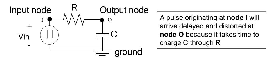
If we focus on the circuit which distorts the pulses produced by Vin, it consists simply of R and C. (Vin is just the time-varying source which produces the input pulse.)
