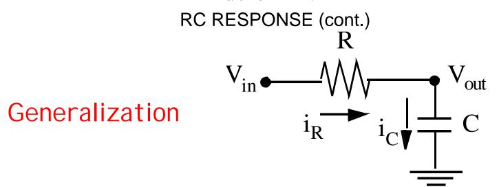
Vin switches at t = 0; then for any time interval t > 0, in which Vin is a constant, Vout is **always** of the form:  $V_{out} = A + Be^{-t/\tau}$
