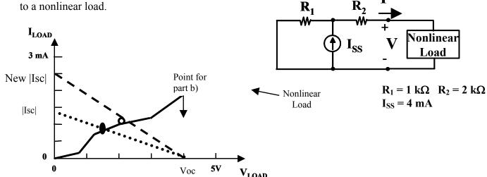
a) (12 points) Find the combination of current I and voltage V that satisfies both the circuit and the load.
