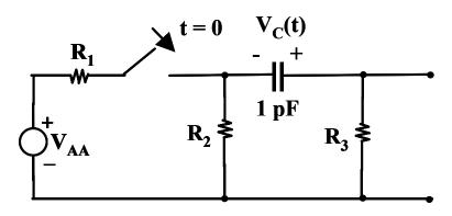
$$\begin{split} R_1 &= 1 k \Omega \quad R_2 = 2 \ k \Omega \quad R_3 = 3 \ k \Omega \\ V_{AA} &= 5 \ V \end{split} \label{eq:controller}$$
