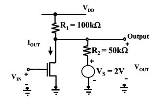
b) (11 points) Now consider the EE 42 device alone with the parameter values given. If  $V_{IN}$  is limited to a range of 0 to 5V and  $V_{OUT}$  is limited to a range of 0 to 5V, what will be the maximum current?
