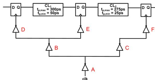
For  $CL_1$ , the max skew added is 20ps ( $t_{skew,D} = +10ps, t_{skew,E} = -10ps$ ), so:
