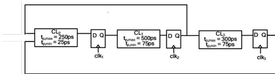
Again, we will use  $clk_1$  as a reference and we will define  $t_{skew1} = t_{clk2} - t_{clk1}$  and  $t_{skew2} = t_{clk3} - t_{clk1}$ . Note that both  $t_{skew1}$  and  $t_{skew2}$  could be positive or negative.
