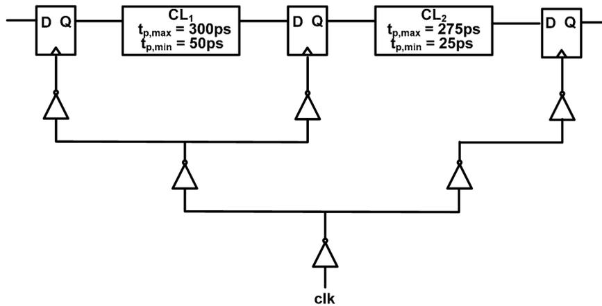
what combination of clock skew causes the worst-case. Each inverter can vary by  $\pm 10ps$ .  $CL_1$  has the max delay, but note that its clocks come from a balanced tree, so it only picks up skew from the last stage (inverters D and E). On the other hand,  $CL_2$  picks up skew from the two last stages (inverters B,E,C,F). In this case, we need to check both cases since it is not immediately clear which one will be critical.
