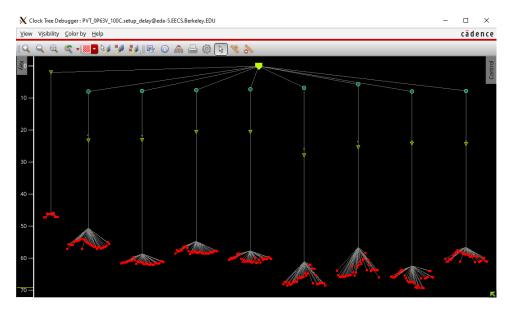
The red dots are the "leaves", the green triangles are the clock buffers, the blue dots are clock gates (they are used to save power), and the green pin on top is the clock pin or the clock "root". The numbers on the left side denote the insertion delay in ps. So, in this view, the tree is upside down, but you get the point.
