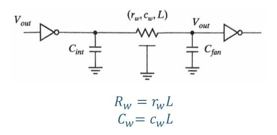
$t_p = 0.69R_{dr}C_{int} + 0.69R_{dr}C_w + 0.38R_wC_w + 0.69R_{dr}C_{fan} + 0.69R_wC_{fan}$ = 0.69(R<sub>dr</sub>(C<sub>int</sub> + C<sub>w</sub> + C<sub>fan</sub>) + R<sub>w</sub>C<sub>fan</sub>) + 0.38r<sub>w</sub>c<sub>w</sub>L<sup>2</sup>
