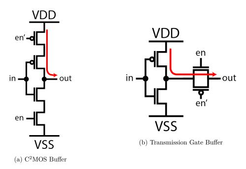
Current paths in both tri-state buffer topologies. Note the two series devices.
