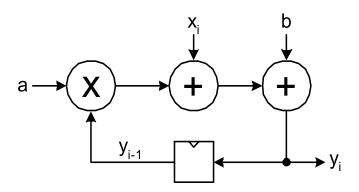
Reorder to shorten the feedback loop and try putting register after multiply:
