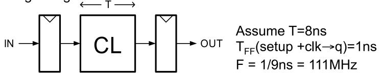
Cut the CL block into pieces (stages) and separate with registers:
