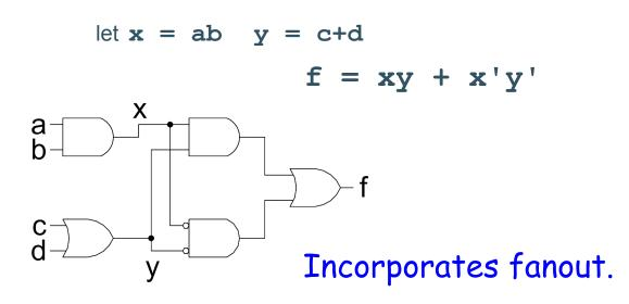
No convenient hand methods exist for multi-level logic simplification:
