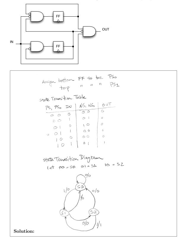
(b) (5 points) Draw the state transition diagram for a *Moore style* finite state machine with the following behavior: The FSM has a single 1-bit input and a single 1-bit output. A reset signal, RST, puts the FSM into an initial state. From there it looks for consecutive input occurrences of 01 and outputs a 1 after the second occurrence, and then on subsequent *contiguous* occurrences. For instance below is a typical input/output sequence:
