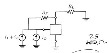
(d) (10 points) Assume a shunt feedback resistor of value  $R_F = 1 \text{ k}\Omega$  is added to the circuit. Calculate  $HD_2$  under this condition. Assume  $R_F \gg R_{in}$ .
