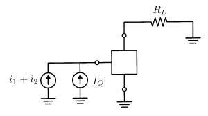
(c) (10 points) For the circuit shown above, calculate the  $IM_3$  at low frequency for two current input signals at 100 MHz and 101 MHz of magnitude 100  $\mu$ A. The circuit is biased as shown with  $I_Q=2\,\mathrm{mA}$ .
