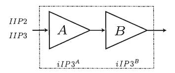
(d) (10 points) Calculate the  $iIP_3$  of the overall amplifier and find the maximum input signal allowed if we desire  $IM_3 > 50$ dBc. The power gain of the first amplifier  $G_A = 17$ dB, the  $iIP_3^A = -11$ dBm, whereas the second amplifier has a gain  $G_B = 50$ dB, and an  $iIP_3^B = +12$ dBm. Note: You may neglect second-order interaction and assume all stages are matched.
