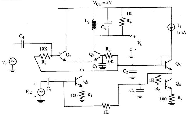
$V_{L0}$  is a local oscillator voltage with frequency 110 MHz and zero-peak amplitude of 60 mV.  $C_1$ ,  $C_2$ ,  $C_3$ ,  $C_4$  and  $C_5$  are large capacitors. The IF tank  $L_2$  -  $C_6$  -  $R_4$  has Q = 20 and is tuned to 10 MHz. Device data:  $\beta = 100$ ,  $V_A = \infty$ , rb = 0
