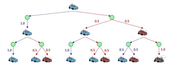
The green nodes represent q-states, where an action has been taken from a state but has yet to be resolved into a successor state. It's important to understand that agents spend zero timesteps in q-states, and that they are simply a construct created for ease of representation and development of MDP algorithms.
