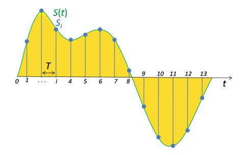
The Waveform Audio File Format encodes a sampled sound wave
