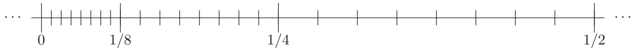
Figure 6.1: Non-negative 3-bit floating-point numbers near 0, showing how the spacing expands as the numbers get bigger. Each tick mark represents a floating-point number. Assume that the minimum exponent is -4 , so that the most closely spaced tick marks are 2^{-6} = 1/64 apart.
