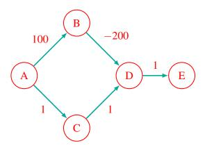
For this graph, if we ran Dijkstra's starting from A, then we would get the incorrect shortest path to E since we would choose the bottom path through C instead of the top path through B.
