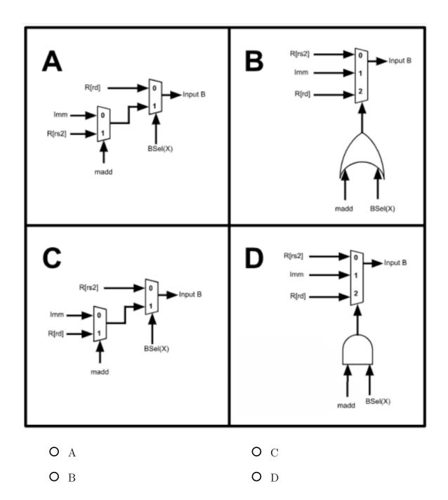
(d) Fill in the correct values for the control signals below to correctly execute a madd instruction. Assume other control bits have been done for you and are correct. For ALUSel, please write an operation name (ie. add) not a numeric value. For RegWEn and WBSel, use integer, decimal numbers.
