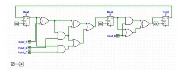
We have a register clk-to-Q time of 5ps, a hold time of 2ps, and a setup time of 3ps. AND and NAND gates have a delay of 5ps, OR and XOR gates have a delay of 6ps, and NOT gates have a delay of 1ps. Assume that our inputs A, B, C, and D arrive on the rising edge of the clock.
