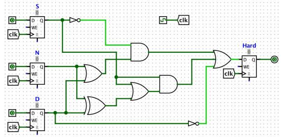
You are given that all logic gates have a propagation delay of 5ps, the register clk-to-q delay is 3ps, the register hold time is 11ps, and the setup time is 8ps. What is the critical path delay of this circuit?
