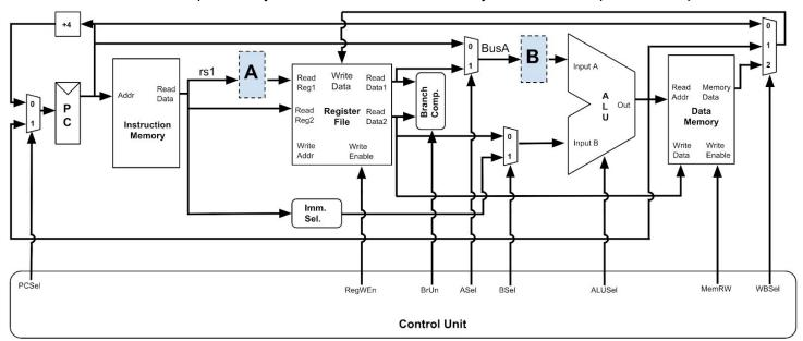
For Parts A and B, please **clearly circle** the correct hardware that would fill their respective dashed boxes above. For Part C, **circle** all the ALUSel operations that could be used by the **luip** instruction in the ALU unit.
