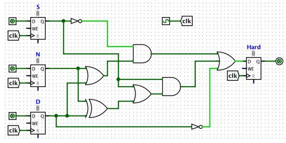
You are given that all logic gates have a propagation delay of 5ps, the register clk-to-g delay is 3ps, the register hold time is 11ps, and the setup time is 8ps. What is the critical path delay of this circuit?
