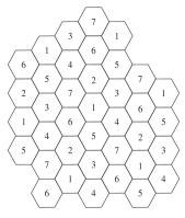
Frequency reuse is poor in narrowband systems because of lack of interference averaging.
