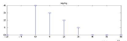
a. Sketch the finite-length sequence y[n] whose six-point DFT is  $Y[k] = W_6^{4k} X[k]$ , where X[k] is the six-point DFT of x[n].
