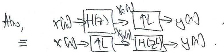
$$Y(\omega) = X_a(\omega L) = H(\omega L) X(\omega L)$$
