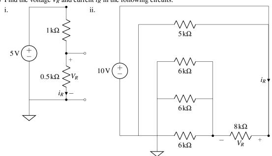
(a) Find the voltage  $V_R$  and current  $i_R$  in the following circuits.
