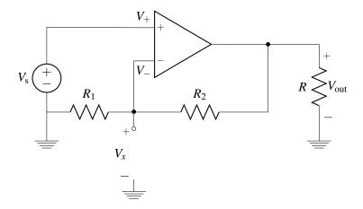
(b) Using your solution to part (a), calculate the limits of  $V_{\text{out}}$  and  $V_x$  as  $A \to \infty$ . Do you get the same answers if you apply the golden rules  $(V_+ = V_- \text{ when there is negative feedback})$ ?
