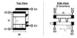
(c) Using the same assumptions as part (b), if you drove terminals  $E_3$  and  $E_4$  with a 1mA current source (as shown below) but left terminals  $E_1$  and  $E_2$  open-circuited, what is the voltage you would measure across  $E_4 - E_3$  (i.e.  $V_{E4-E3}$ )?
