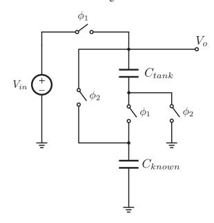
In this circuit,  $C_{\text{tank}}$  is the total tank capacitance that you calculated earlier.  $C_{\text{known}}$  is some fixed and known capacitor. Find the voltage  $V_o$  in phase  $\phi_2$  as a function of the height of the water. Note that
