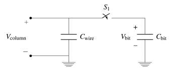
(d) The minimum voltage the readout circuit needs to reliably detect a "1" in a DRAM cell is 0.4V. Considering  $C_{\rm bit} = 18 fF$ , and using the same dimensions provided in part b) for the wires, what is the maximum number of cells that can be stacked together on to a single DRAM column while still meeting this minimum voltage requirement for the readout?
