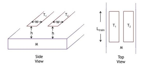
Assuming that the entire train is at a uniform height above the track and ignoring any fringing fields (i.e., all capacitors are purely parallel plate), as a function of  $L_{\text{train}}$  (the length of the train), W (the width of  $T_1/T_2$ ), and h (the height of the train off of the track), what is the capacitance between  $T_1$  and M? How about the capacitance between  $T_2$  and M?
