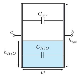
The width and length of the tank are both w (i.e. the base is square) and the height of the tank is  $h_{tot}$ .
