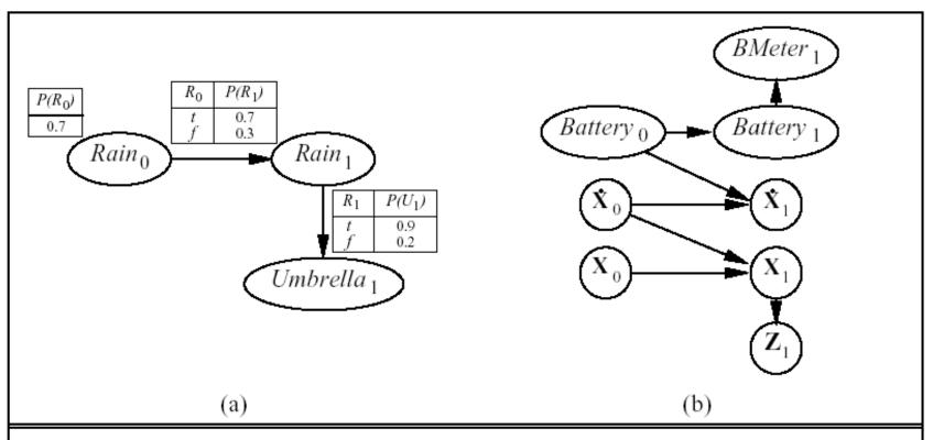
**Figure 15.11** (a) Specification of the prior, transition model, and sensor model for the umbrella DBN. All subsequent slices are assumed to be copies of slice 1. (b) A simple DBN for robot motion in the X–Y plane.
