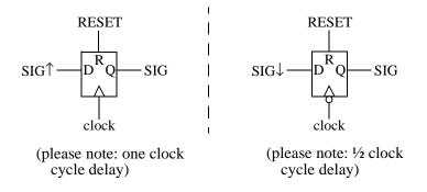
Assume that the clock is slow, say 1 MHz, but that outputs may be delayed from 0 to 100 ns because of routing delays. A BUFGS is used to prevent clock skew.
