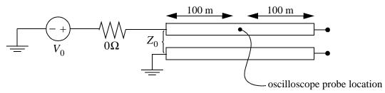
$V_0$  switches at time t = 0, as shown. Sketch the voltage seen on the oscilloscope for  $0 < t < 10 \mu s$ . ( $V_0$  is initially at 5V,  $-\infty < t < 0$ .)
