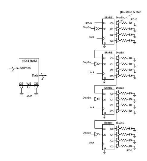
[11 pts.] a) Complete a detailed block diagram of the data path for the LED PWM Display, using up to three CB4RE synchronous binary counters, one COMPM4 4-bit magnitude comparator, and one COMP4 identity comparator. Note that CB4RE has both a TC output =  $Q_3 \cdot Q_2 \cdot Q_1 \cdot Q_0$  and CEO =  $TC \cdot CE$ . Also, SR4RE shifts left.
