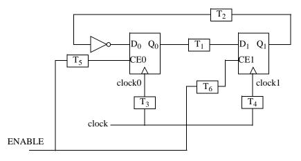
[2 pts.] a) Assuming proper operation, draw the state diagram for the FSM, assuming  $T_3 = T_4 = 0$  ns. Use notation for the state as  $(Q_1 Q_0)$ .
